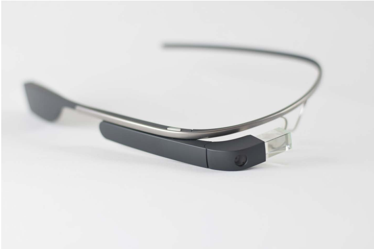
Figure 1. Google Glass, prototypical head-worn smartglasses with in-built sensors, as well as a small screen and a bone conduction speaker to provide a private audio-visual experience. The BPAS integrates Google Glass with a range of assistive science-based modules.
