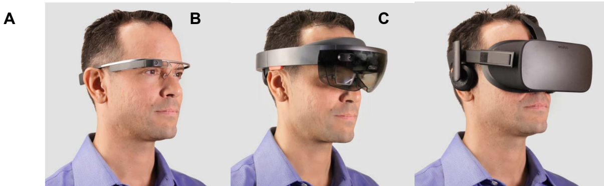
Figure 1. Head-worn Computers or Displays. (A) Glass Explorer Edition (originally known as Google Glass): augmented reality (AR) smartglasses with fully stand-alone onboard computer (weight 42 grams). (B) Microsoft HoloLens: AR headset with fully stand-alone onboard computer and depth camera (weight 579 grams). (C) Oculus Rift: virtual reality (VR) headset display, which must be tethered continuously to a powerful computer to drive it (weight 470 grams). VR headsets and some AR devices are large, heavy, and block the social world considerably. Image depicts study author NS.
